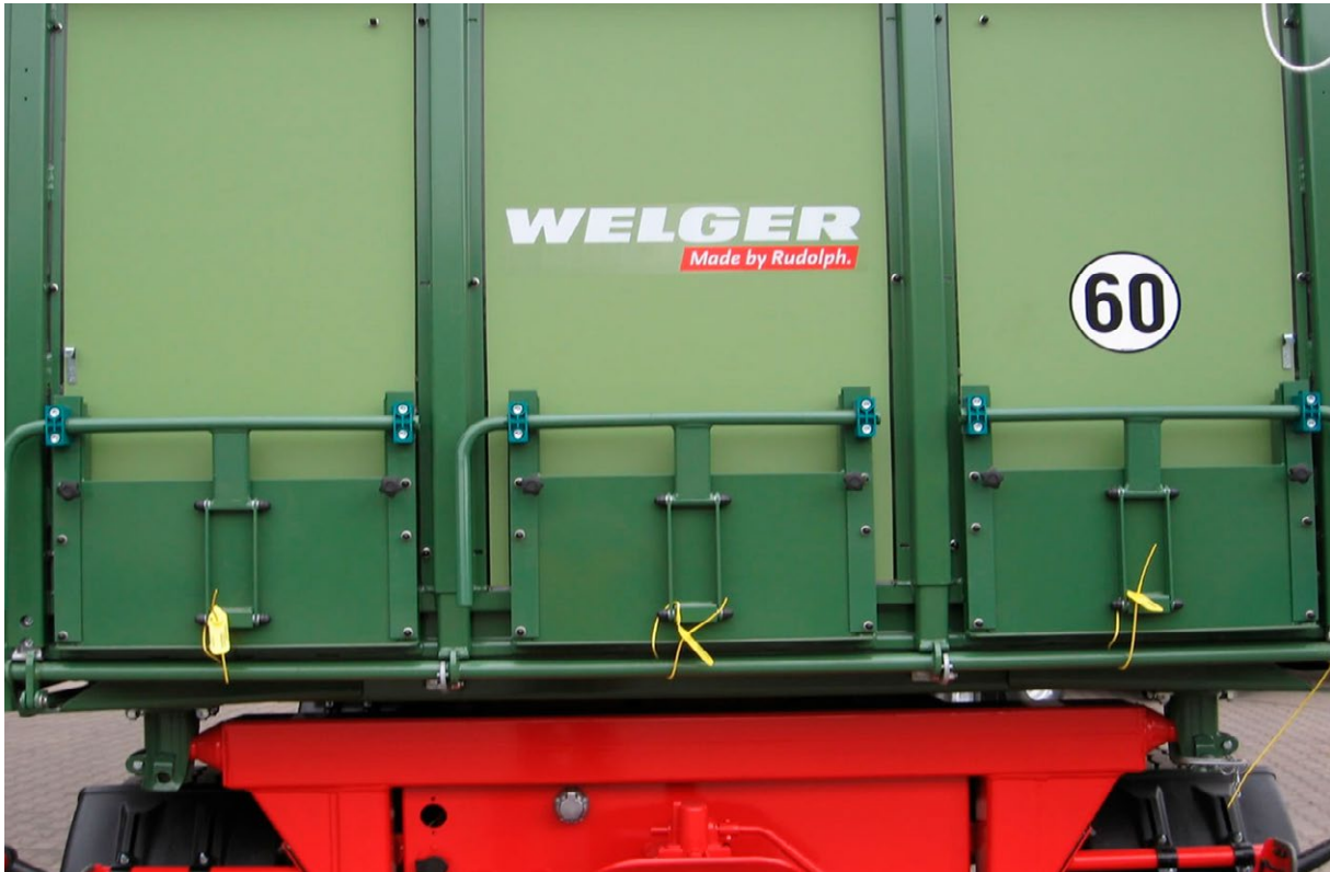
Photo 26: Use of tamper evident seals to close the doors of a bulk vehicle.
