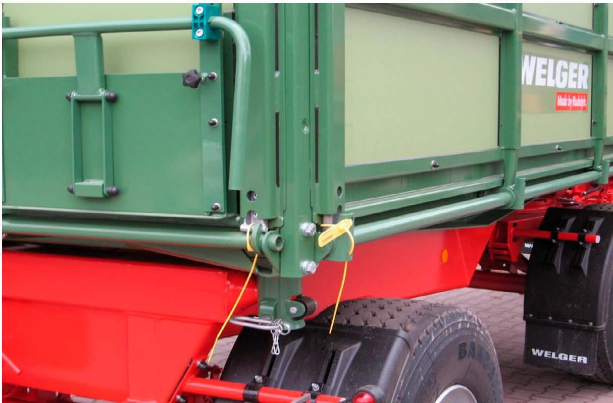
Photo 27: Use of tamper evident seals to close the rear and sides of a bulk vehicle.
